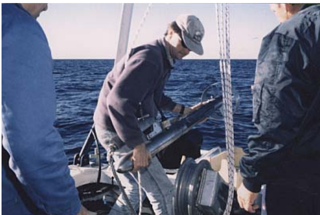
Figure 17: Mr Steve Holtznagel deploying the Department of Land & Water Conservation's side scan sonar, during the remote mapping phase of the project. Photo: David Nutley.
