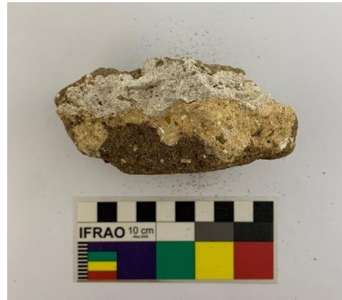
Figure 4.2 Mortar sample with layers of yellow and grey shell lime mortar (BCN17x0228, Context 222)
