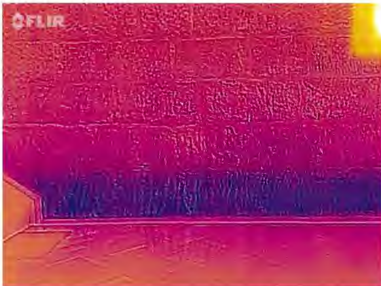
Figure 14 Thermal image of the exposed stonework on the inside of the north wall of Unit 20. Yellow colours are warm (TV at top right, stairs and mat at bottom left), deep purple is cool. Note how the bedrock is coolest and how there is a reasonably crisp distinction in temperature between the bedrock and the made stonework above. Part of the reason that the bedrock is cooler is because of evaporation of moisture into the room.
