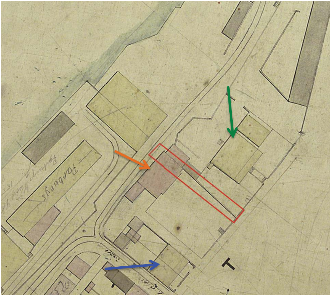
Figure 2.3 Part of an 1865 trigonometrical survey of Sydney. Approximate location of study site outlined in red. Orange arrow points to John Nicholson's Durham residence while the blue arrow indicates the terraces at 21-23 Lower Fort Street (still standing), green arrow points to Walker's residence (now incorporated into the terrace 7-9 Lower Fort Street). Construction material key: Pink/red = brick, Beige/yellow = stone, Grey = wood, Blue = iron. Historical Atlas of Sydney (1865, Section A2)
